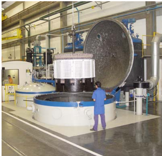
VPI System Diameter: 3.5 m Height: 6 m
